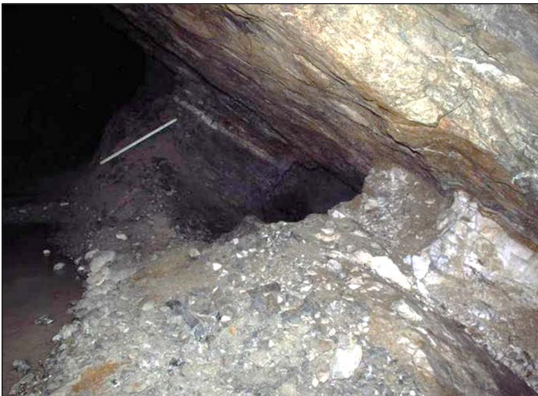
Figure 6-16 Main Vein reducing in thickness from 110 cm in the foreground to 15 cm over a distance of only 4 m in the 390 Level East reef drive (source: SRK ES 2016)
