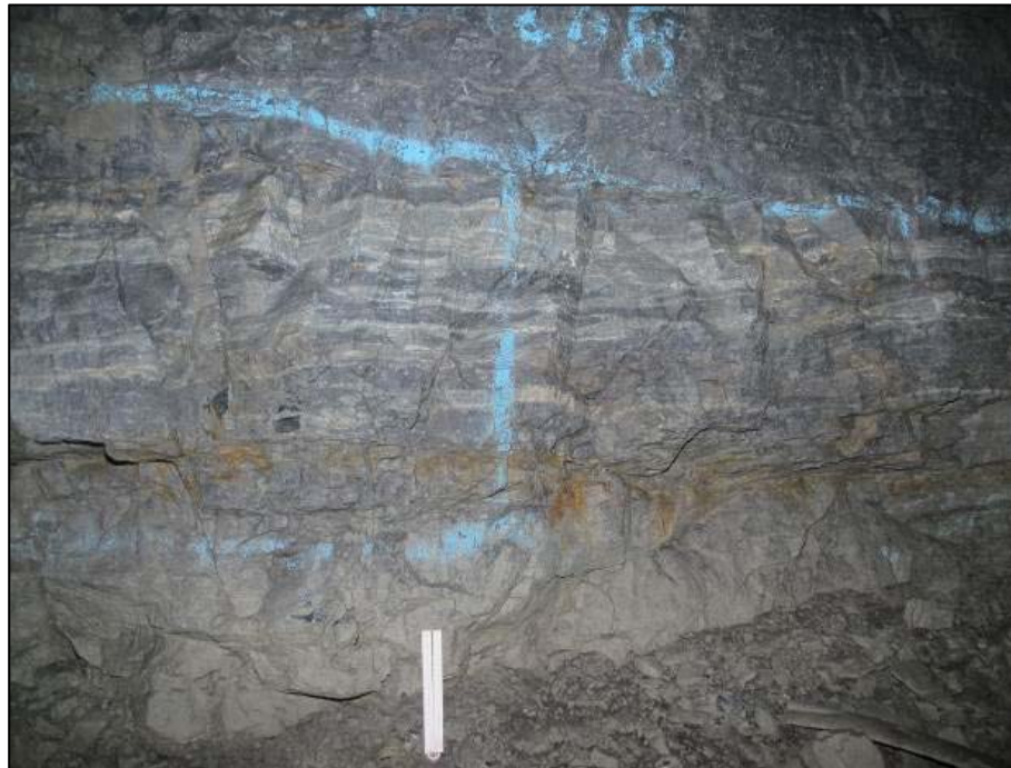
Figure 8-10 SRK ES interprets these as FW lithologies in a drive that has deviated from the MV structure. The blue lines indicate that they have been marked and sampled as the MV by previous operators. 600 Level Target Block West (source: SRK ES 2016)
