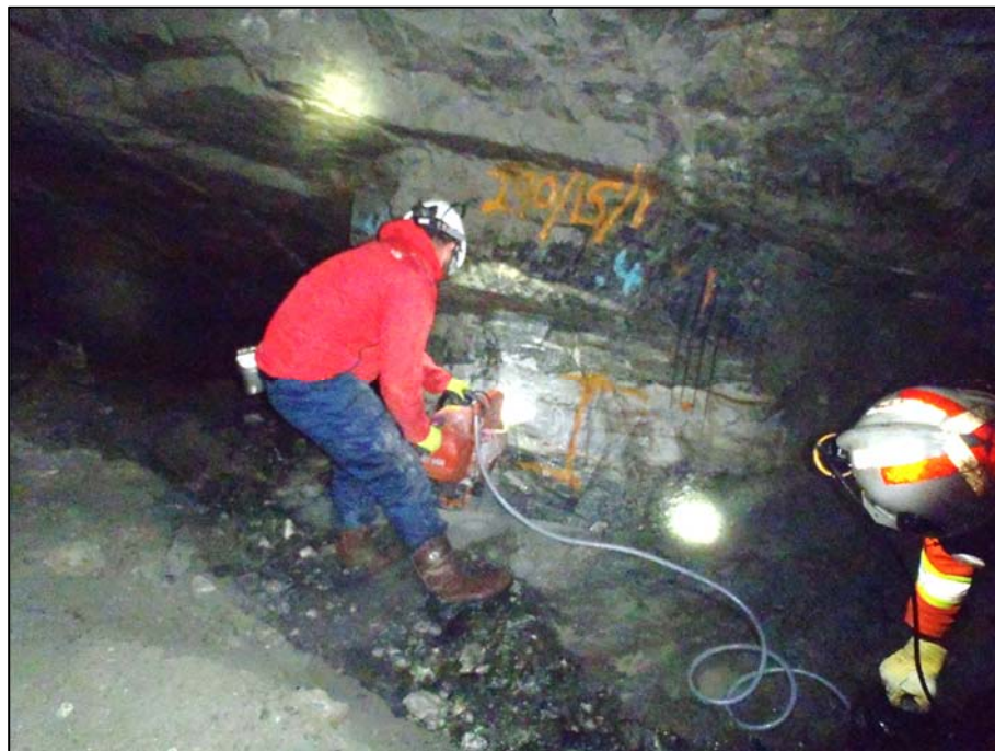
Figure 8-16 Cutting out the sample using a diamond-bladed rock saw. Note the parallel cuts in the hanging wall (source: SRK ES 2016)
