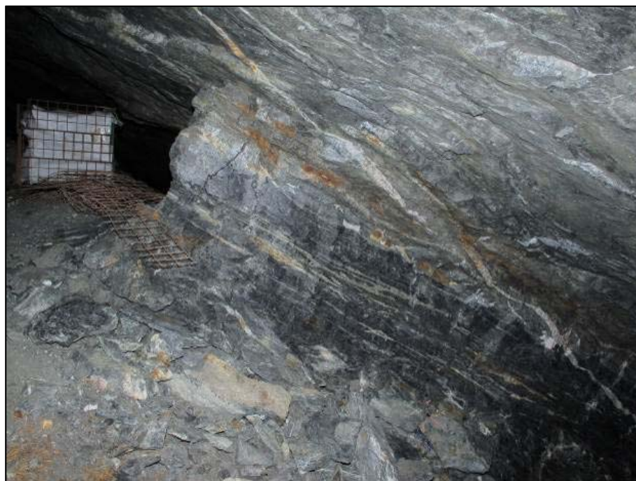
Figure 8-11 FW lithologies in a stope pillar showing parallel veining/alteration that is typically found below the MV. The MV is probably in the HW rocks above (source: SRK ES 2016)
