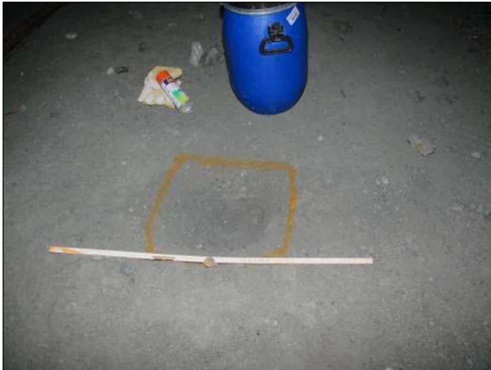
Figure 8-25 Sampling pit dug in 22 cm thick sweepings in the 310 SB Level below the #18 stope (source: SRK ES 2016)
