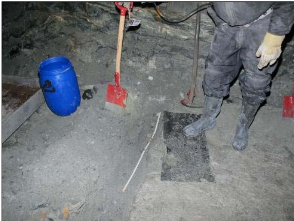
Figure 8-24 Sampling trench dug across 22 cm thick sweepings in the 300 SB Level drive below the #15 stope (source: SRK ES 2016)
