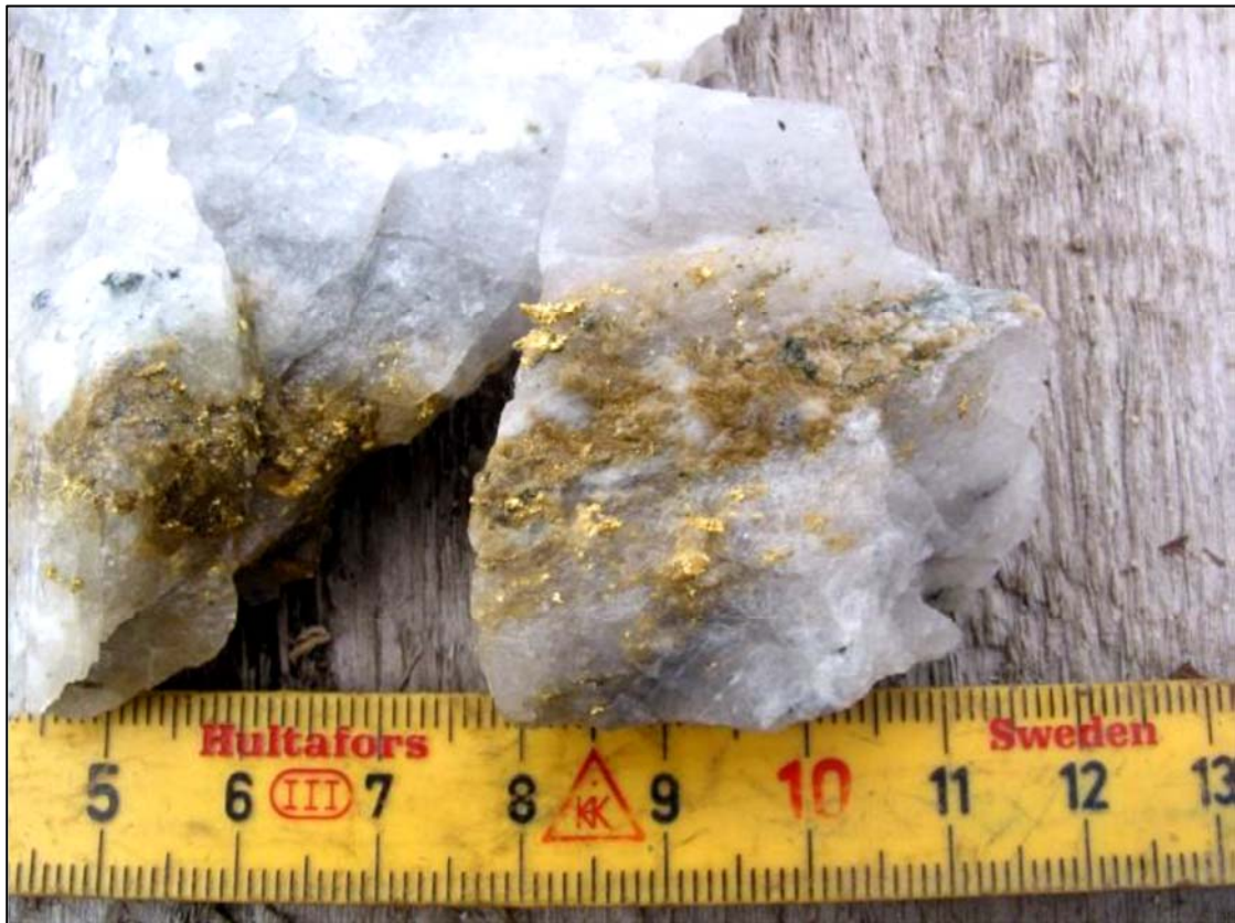
Figure 7-1 High grade gold-quartz vein sample from the Nalunaq Main Vein containing coarse gold (source: Crew Gold Corporation).
