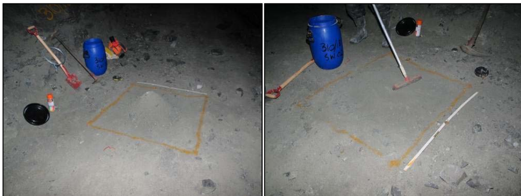
Figure 8-26 Sweepings sampling in 1 m 2 of 5 cm thick material on the 310 SB Level below the #18 stope with material scraped (left image) and then the surface swept (right image). Source: SRK ES 2016
