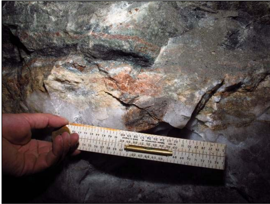
Figure 8-12 Ankerite, epidote and quartz in a FW vein. 350 Level Target Block West (source: SRK ES 2016)
