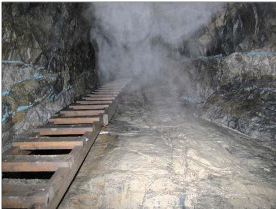
Figure 6-27 580 Level ventilation raise – on an aplite dyke but apparently sampled as shown by blue sampling lines (source: SRK ES 2016)
