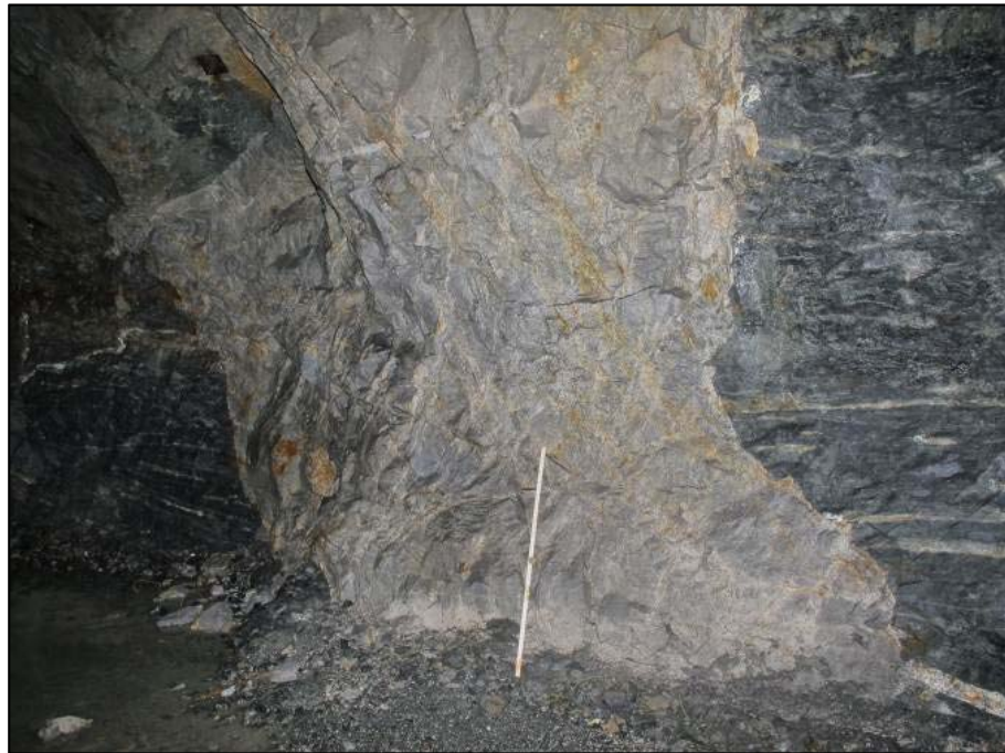
Figure 6-29 Large aplite dyke on the 720 Level Mountain Block West exploiting a fault (MV displaced) (source: SRK ES 2016)
