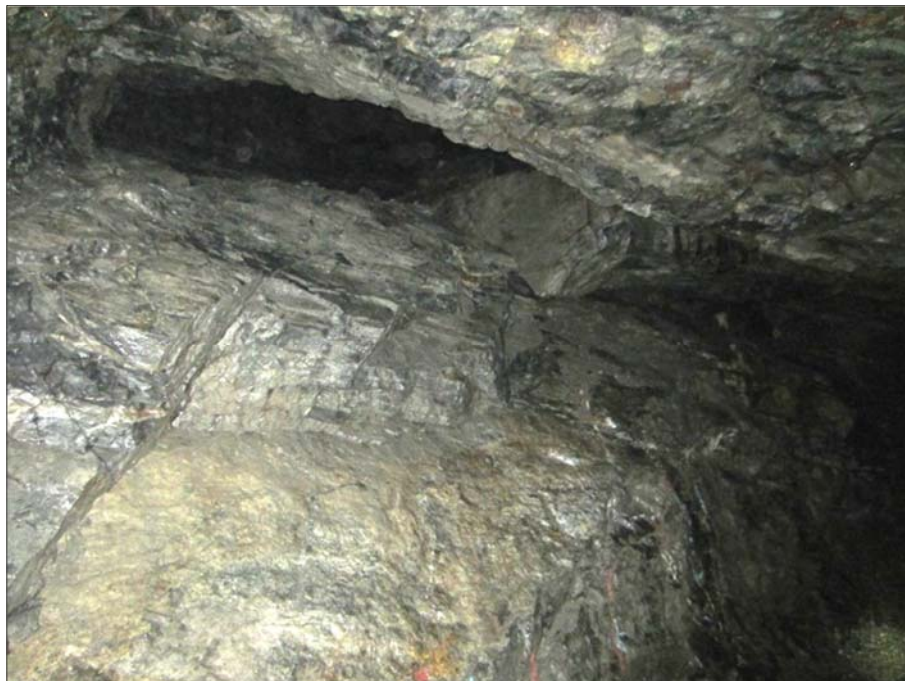
Figure 23-1 Marginally-stable dislodged rock block in stope 490-07 above a stope drive (source: SRK ES, 2016)
