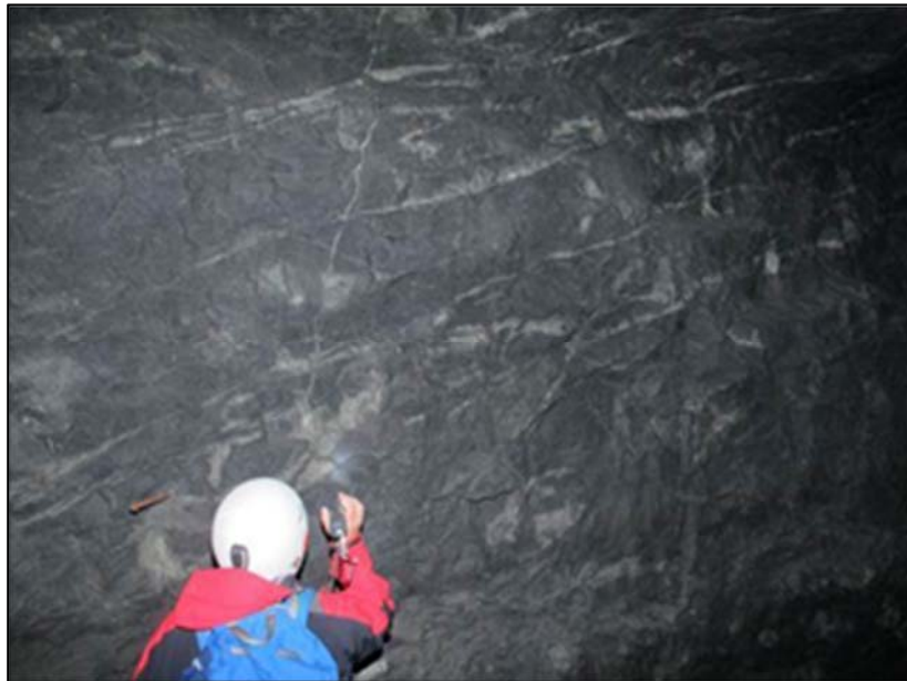
Figure 6-7 Typical FW lithology showing conjugate veins and stringers of calc-silicate alteration (source: SRK ES 2016)
