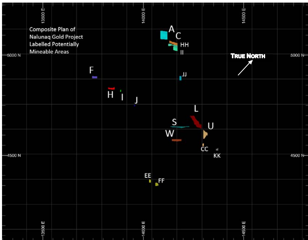
Figure 8-23 Resulting potentially mineable areas with existing excavations removed for clarity (source: SRK ES 2016)
