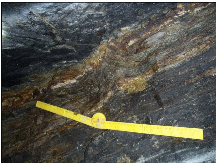
Figure 6-21 Small ramp-like structure resulting from thrusting on the MV structure (devoid of veining at this location). 600 Level East Mountain Block (source: SRK ES 2016)
