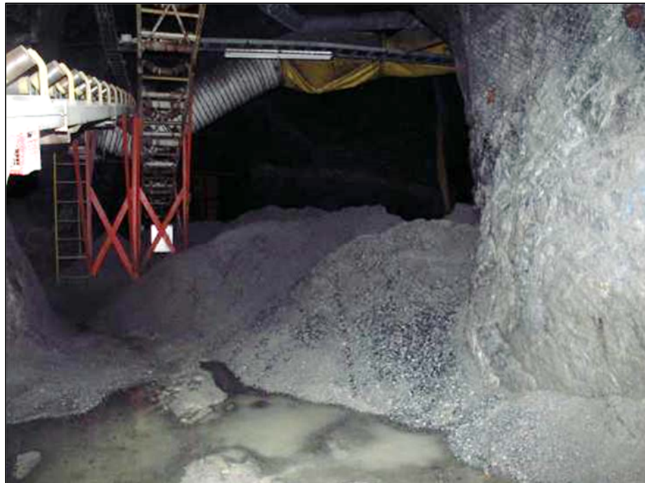
Figure 8-27 Example of accumulated material, possibly gold-bearing, beneath conveyor belts in the processing plant (source: SRK ES 2016)
