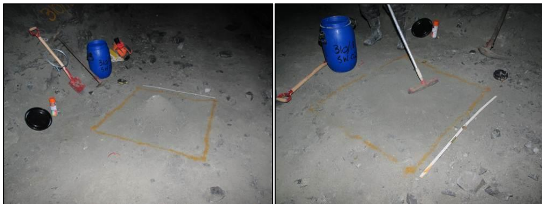
Figure 5-44: Sweepings sampling (300 18 SW02) in 1 m 2 of 5 cm thick material on the 310 SB Level below the #18 stope with material scraped (LHS) and then the surface swept (RHS)(SRK ES, 2016)
