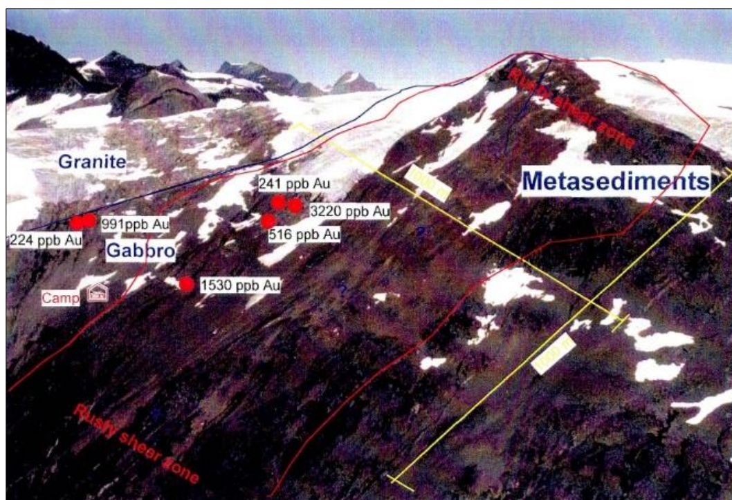
Figure 10-6: Oblique aerial photo of Jokum's Shear showing the upper part of the shear zone and locations of gold-anomalous grab samples (Swiatecki, 1997)
