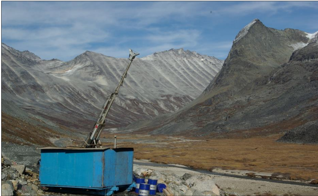
Figure 5-14: Skid-mounted rig drilling from the Nalunaq Mine road in 2017 (AEX, 2018)
