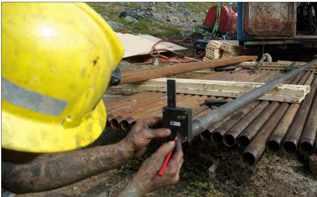
Figure 5-15: Marking the bottom of hole line on drill core using the Reflex ACT tool in 2017 (AEX, 2017)
