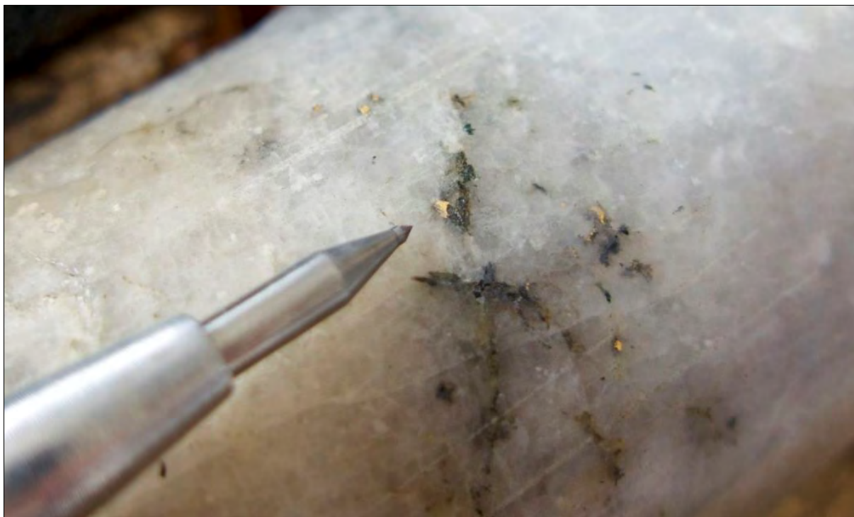
Figure 5-21: Quartz vein containing clinopyroxene stringers and visible gold interpreted to be MV of Nalunaq Mine (AEX, 2018)
