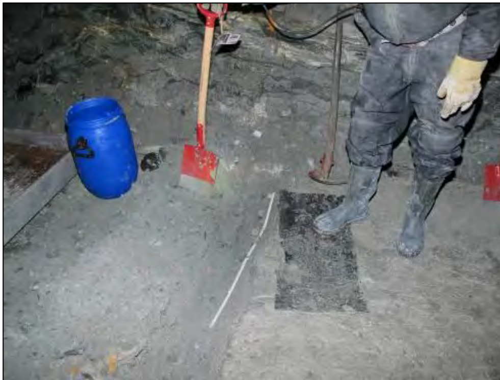
Figure 5-43: Sampling trench dug across 22 cm thick sweepings in the 300 SB Level drive below the #15 stope (SRK ES, 2016)
