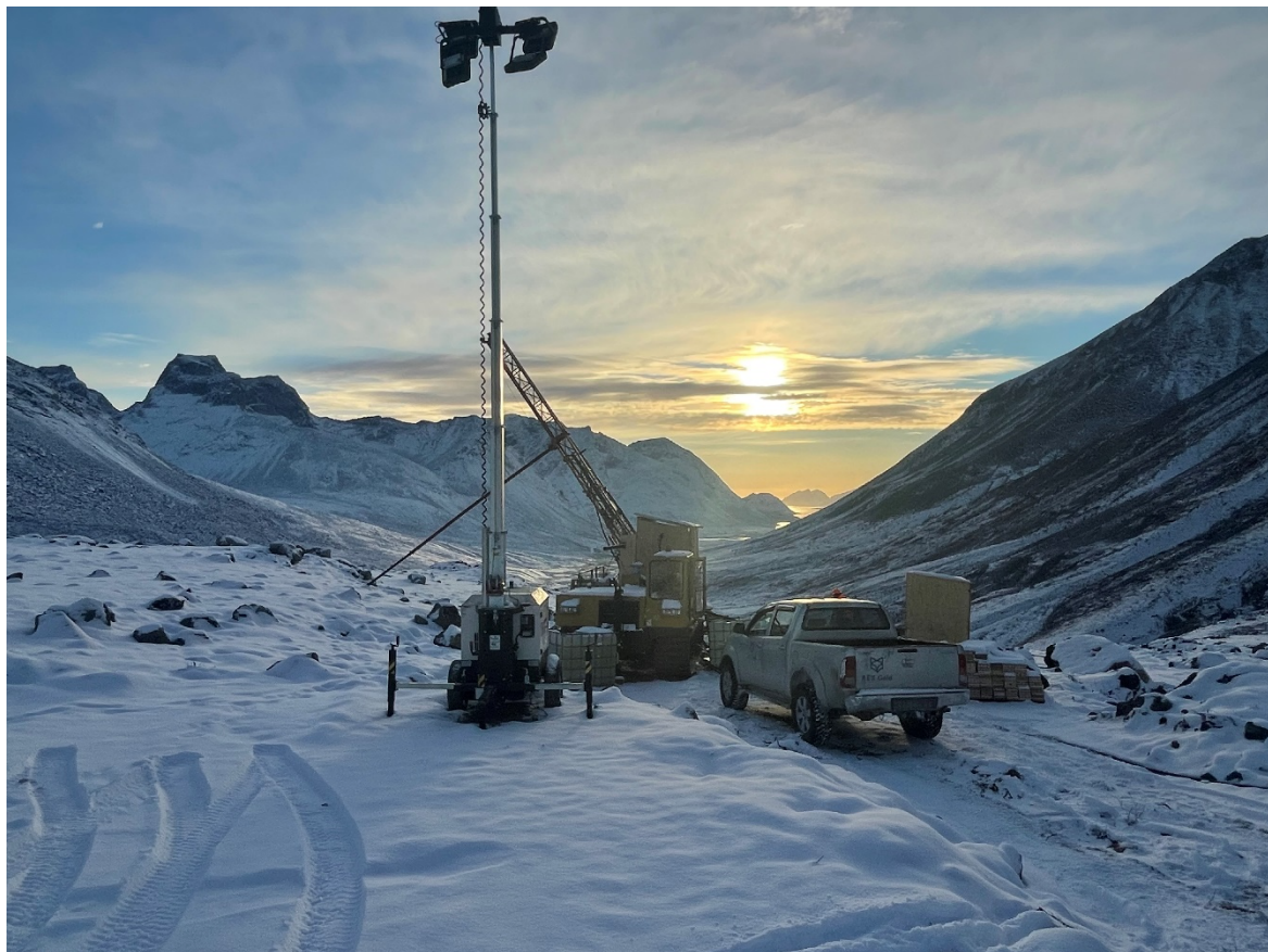
One of four winterised core rigs in operation at Nalunaq
