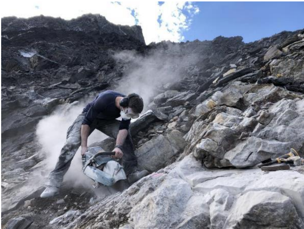
Figure 4. Surface channel sampling on the Main Vein exposed within the Mountain Block
