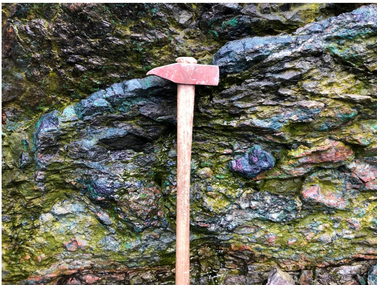
Figure 2. Skarn hosted massive sulphide mineralisation observed at Josva – 11.6% Cu over 50cm
