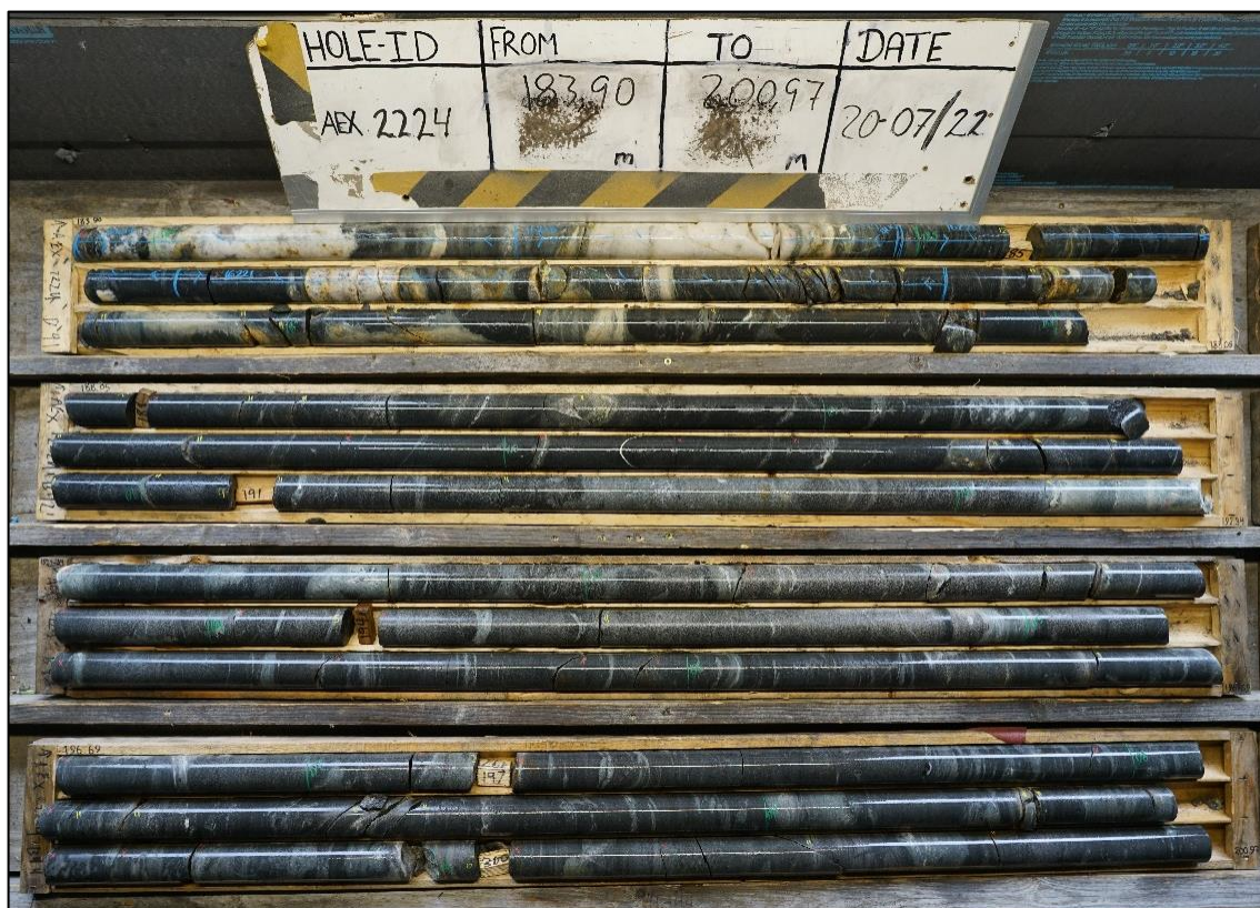
Figure 6-19: Main Vein (top row) with fine-grained banded amphibolite in the hanging wall and immediate footwall, followed by 13m of medium-grained dolerite in the footwall
