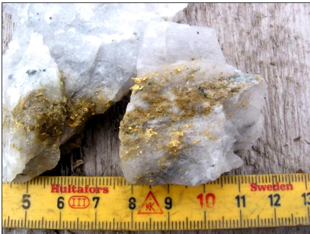
Figure 7-1: High grade gold-quartz vein sample from the Nalunaq Main Vein containing coarse gold (Image Source: Crew Gold Corporation).
