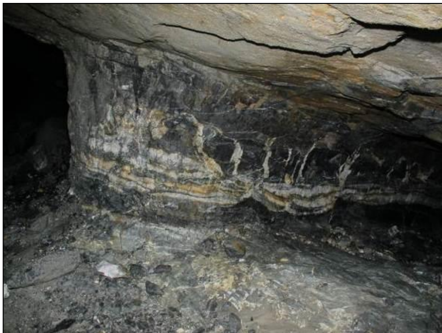
Figure 6-21: The Main Vein structure in the Target Block exhibiting quartz-filled tension gashes perpendicular to the Main Vein (Image Source: SRK ES, 2016)
