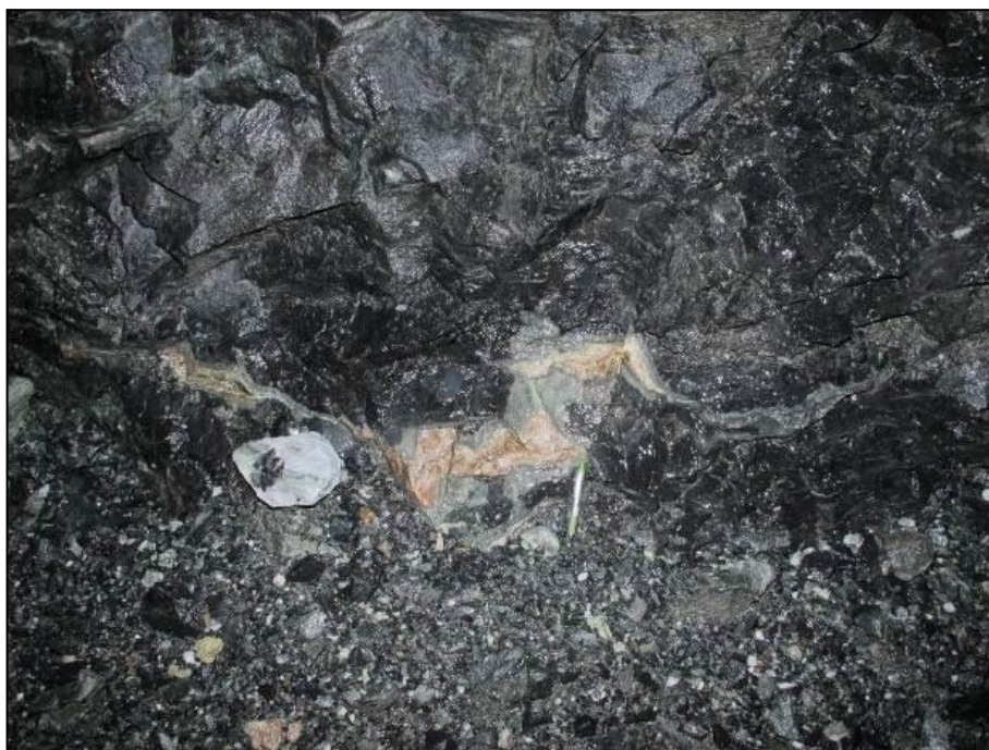
Figure 6-10: Dark coarse-grained meta-dolerite in the HW showing some garnet-epidote alteration. This is less common in the HW than the FW. (Source: SRK ES, 2016)
