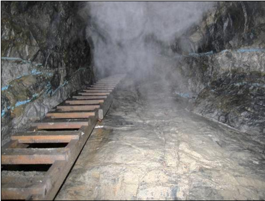
Figure 6-15: 580 Level ventilation raise along on an aplite dyke but apparently sampled as shown by blue sampling lines (Image Source: SRK ES, 2016)
