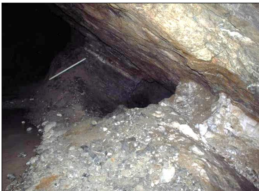
Figure 6-23: Main Vein reducing in thickness from 110 cm in the foreground to 15 cm over a distance of only 4 m in the 390 Level East reef drive (Image Source: SRK ES, 2016)
