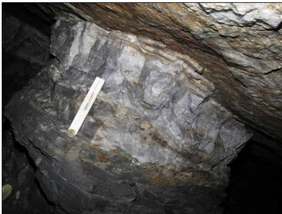
Figure 6-20: Classic form of the Main Vein in the Mountain Block showing grey vitreous quartz. 630 Level, stope number 1 (Image Source: SRK ES, 2016)
