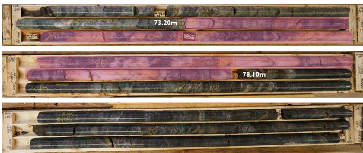
Figure 2: Recovered core from hole NAN2517, 73.20m to 78.10m – 4.90m for 19.60 g/t Au hosted in a complex folded quartz vein between a tuff and volcanic sandstone unit.
