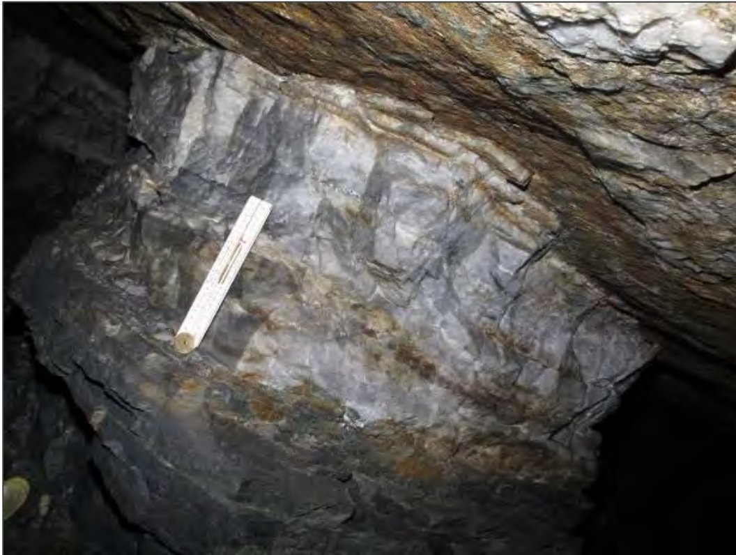
Figure 3-11 Classic form of the Main Vein of the Mountain Block showing grey, vitreous 'bull quartz' (630 Level, Stope #1)
