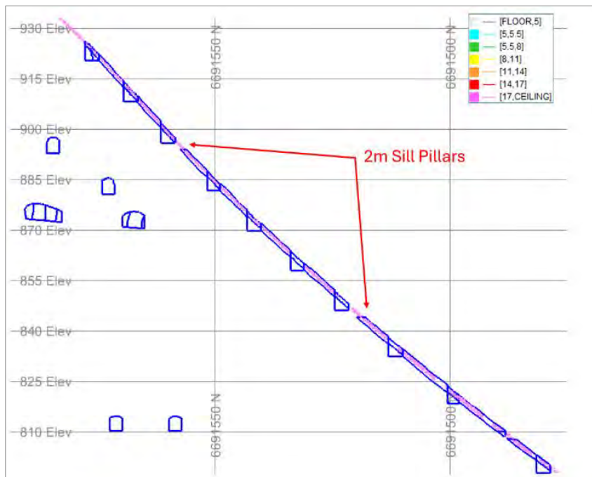
Figure 6-3 Plan view of the Mountain Block mine design showing designed stope extents, pillar positions, and crown pillar boundary
