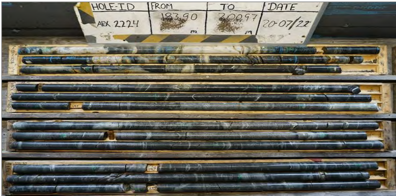
Figure 3-9 Main Vein (upper box) with fine-grained banded amphibolite in the HW and immediate FW, underlain by 13 m of medium-grained dolerite in the FW
