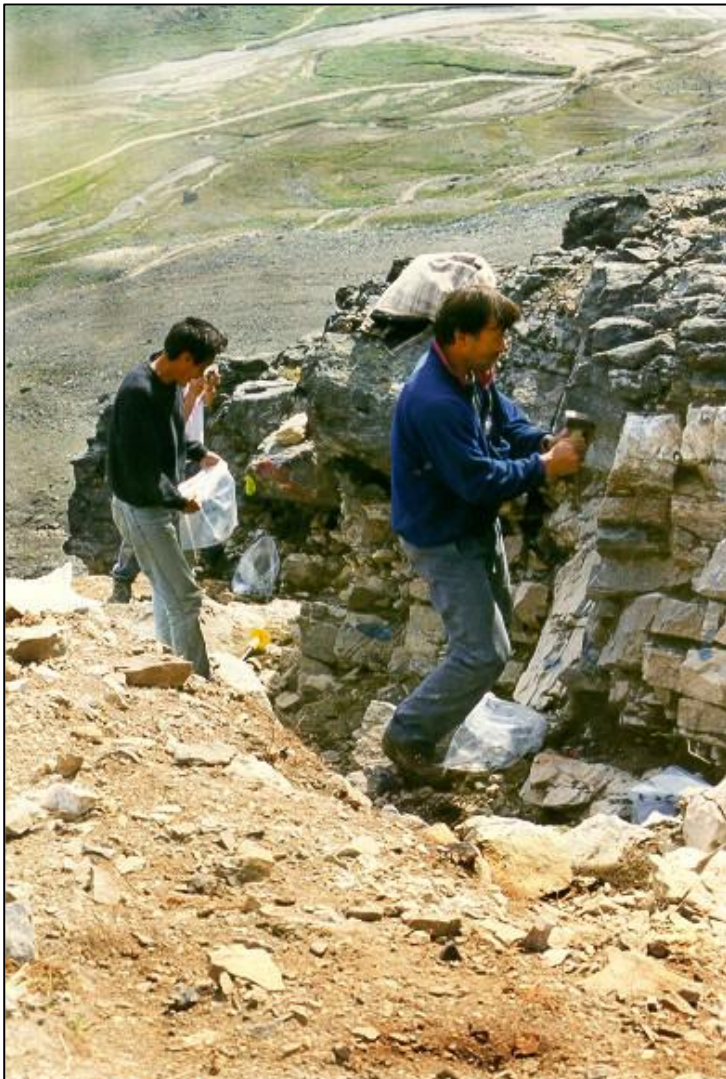
Figure 6-2 Chipping of the surface channel samples at 1 m intervals, after cutting with a diamond blade saw
