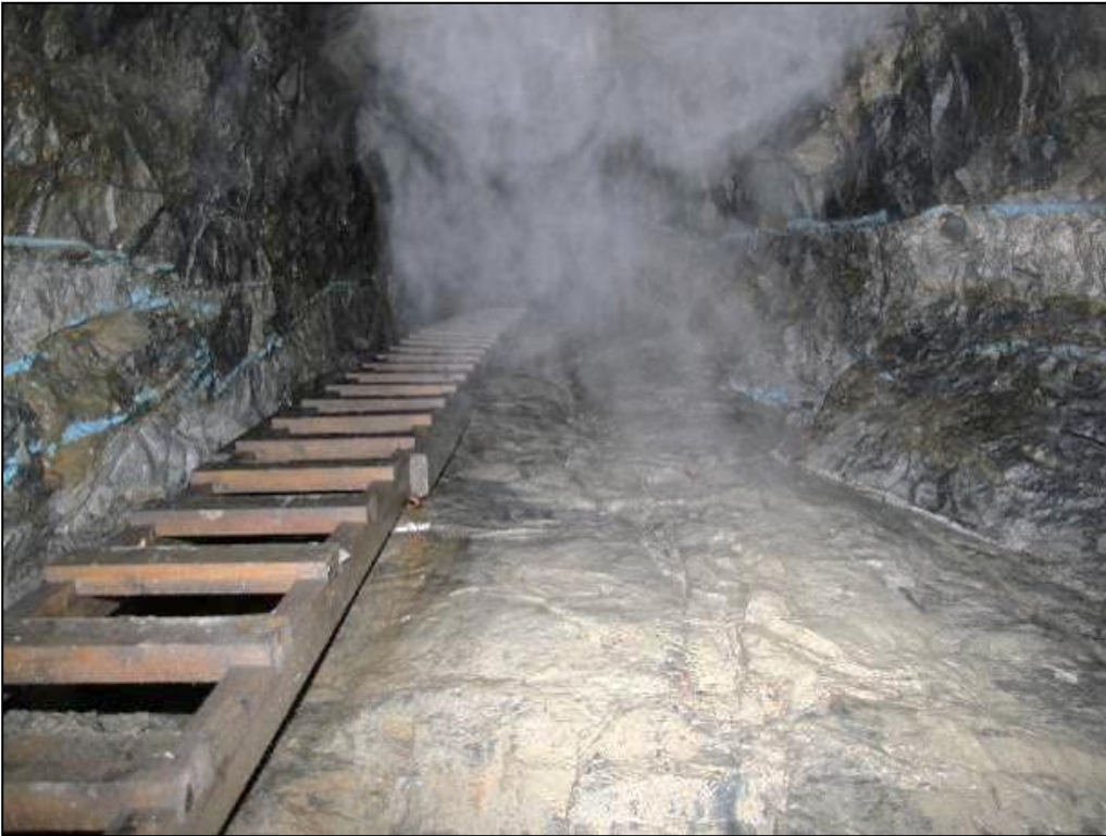
Figure 7-17 580 Level ventilation raise – on an aplite dyke but apparently sampled as shown by blue sampling lines
