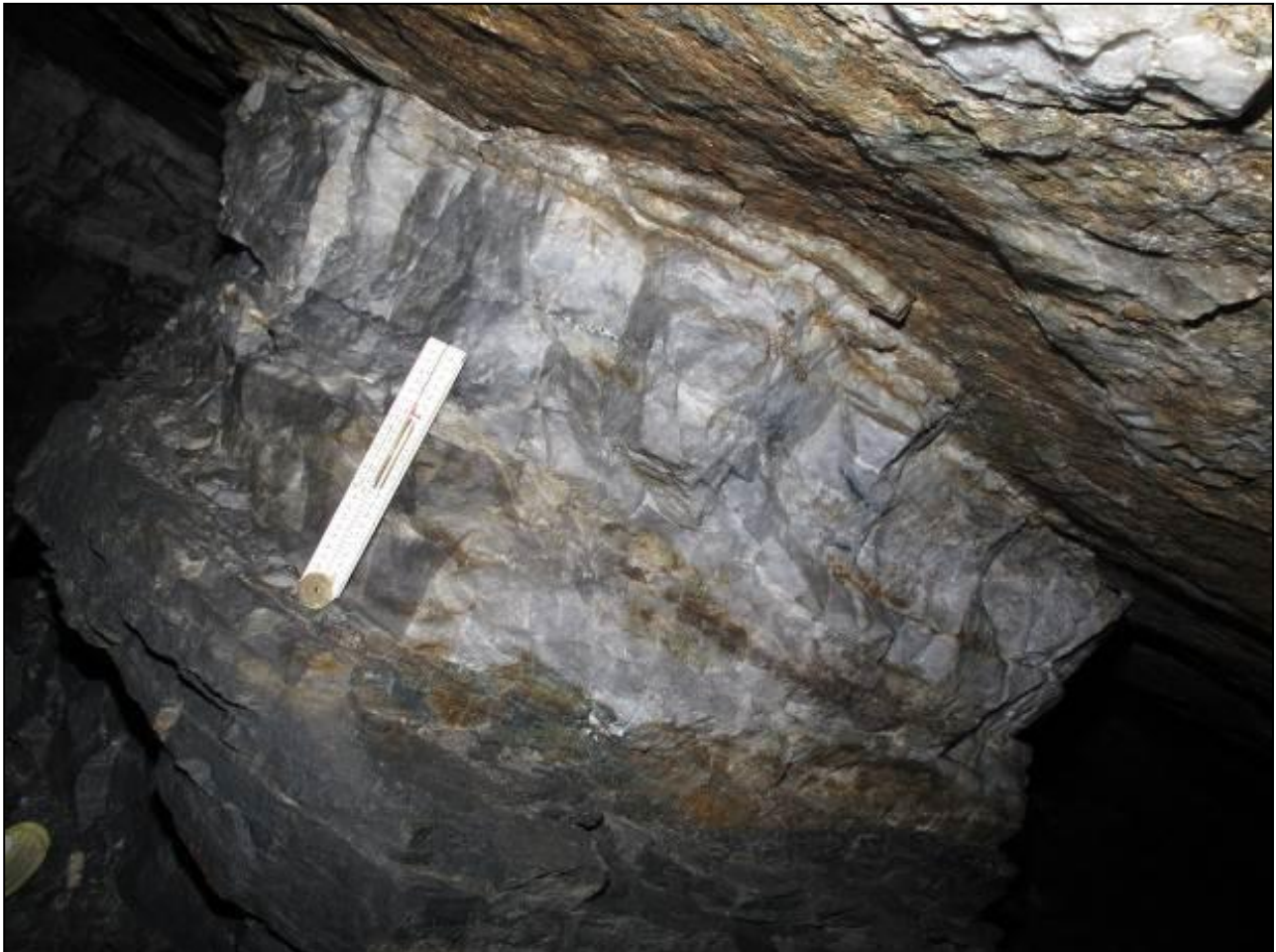
Figure 7-22 Classic form of the Main Vein in the Mountain Block showing grey vitreous quartz (630 Level, stope #1)
