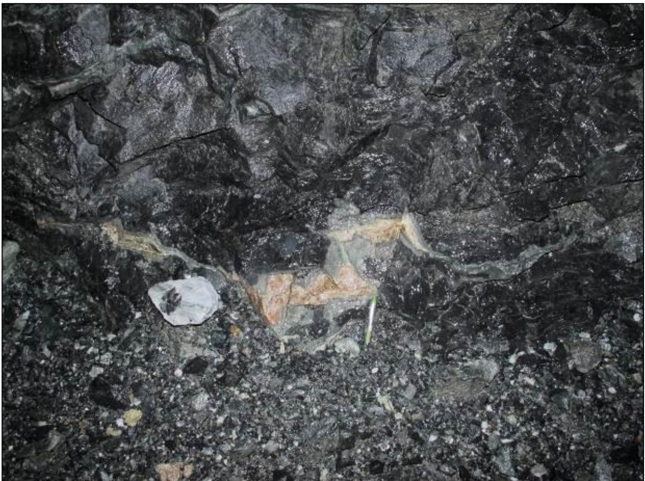
Figure 7-11 Dark coarse-grained meta-dolerite in the hangingwall showing some garnet-epidote alteration; this is less common in the hangingwall than the footwall
