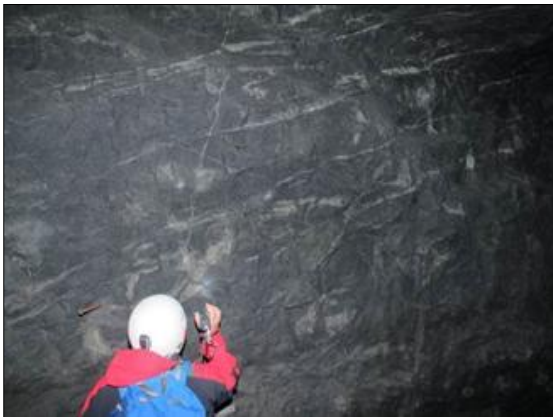
Figure 7-9 Typical footwall lithology showing conjugate veins and stringers of calc-silicate alteration
