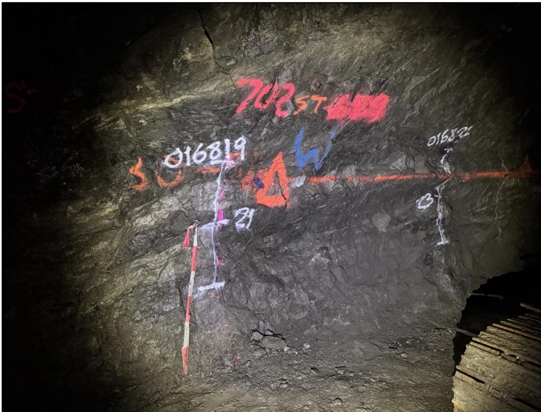
Figure 11-28 Sidewall samples marked up ahead of sampling with a diamond blade saw
