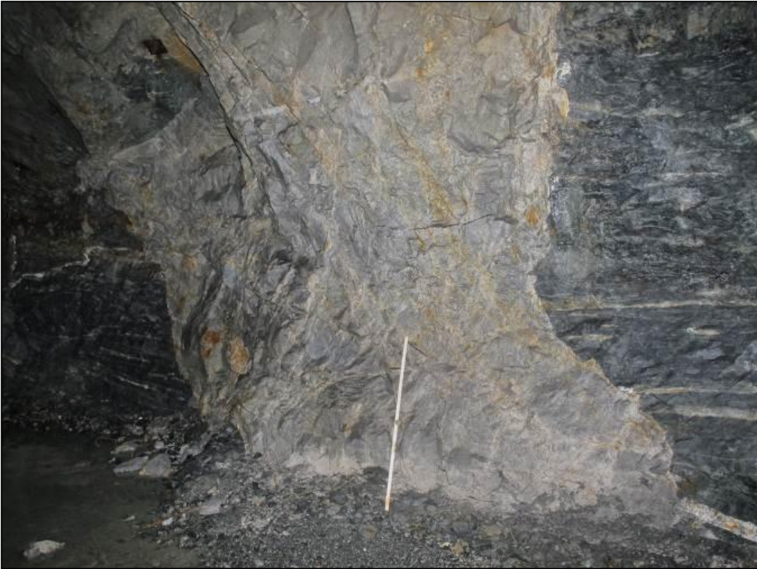
Figure 7-19 Large aplite dyke on the 720 Level Mountain Block West exploiting a fault (Main Vein displaced)
